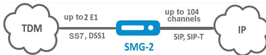
Fig. 1.2—Interfacing of TDM and VoIP Network Signalling and Media Streams Using SMG-2
