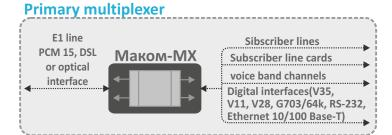
In Termination Multiplexer mode the equipment enables to connect devices via analoq and digital interfaces and also to connect to remote devices by E1 lines , PCM-15 or optical cable according to TDMoIP technology.
