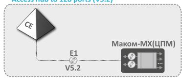
Central processor (ЦПМ) application enables Маком-МХ to arrange access hub from telephone exchange (БКП-М) or other exchange by V5.2 protocol.
