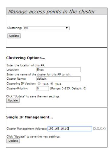
To edit the settings in **«Clustering Options»** section, switch cluster mode to **«Off»** state. In **«Clustering Options»** menu, perform the following configuration:
